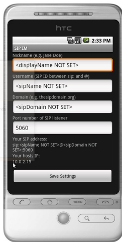
Figure 2 SIP configuration UI on Android
